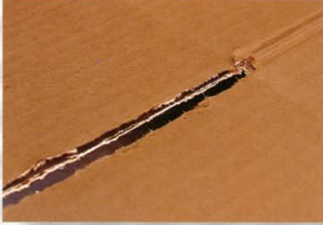
Recycled paper is very difficult to slot with conventional slotters.
