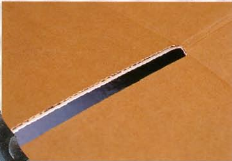
Zenith Cutter serrated male slotters provide cleaner slots and much longer life.
